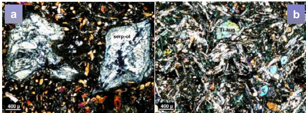
Figure 3.3. a) Serpentine pseudomorphs after olivine. Note that the pseudomorph at the left hand side has been largely resorbed by groundmass. Minerals with higher interference colors in the groundmass are Ti-augite. (Sample GK-1, XPL); b) Augite-phyric metabasalt with relatively larger groundmass plagioclase. The interstices between plagioclase crystals are occupied by Ti-augite, which is distinguished by higher interference colors (Sample OR-41, XPL) (serp-ol: serpentinized olivine; Ti-aug: Ti-augite).
