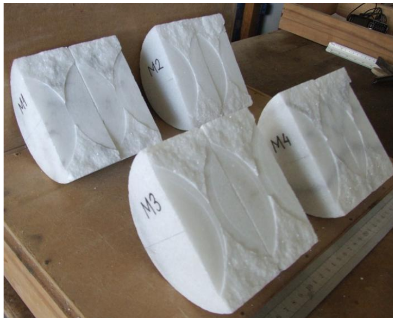
Figure 8. 14 CCNBD specimens after fracturing
