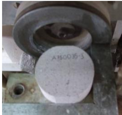
Figure 8. 19 Adjustment to get parallel loading ends
