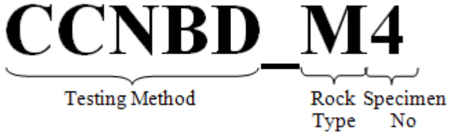
Figure 8. 17 Specimen coding; CCNBD: cracked chevron notched Brazilian disc, A: rock type (A for andesite and M for marble), 4: specimen number
