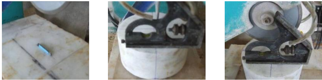
Figure 8. 9 A flat block with knife piece (on the left), horizontal plane measurement perpendicular to notch (on the center) and horizontal plane measurement parallel to notch (on the right)
