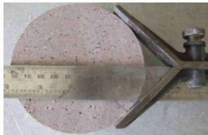
Figure 8. 4 Diametral line drawing with goniometer (on the left) and fixed disc on cutting machine with holding fixture (on the right)
