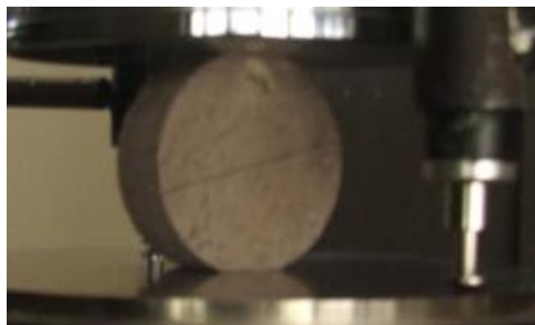
Figure 8. 20 FBD specimen under loading
