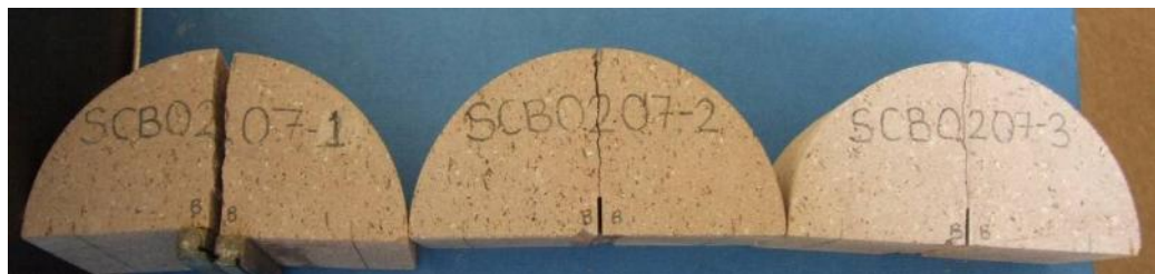
Figure 8. 6 Semi-circular bending specimens after cracking and fracturing
