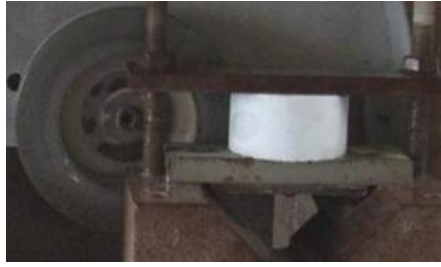
Figure 8. 18 Flattening loading end with grinding machine
