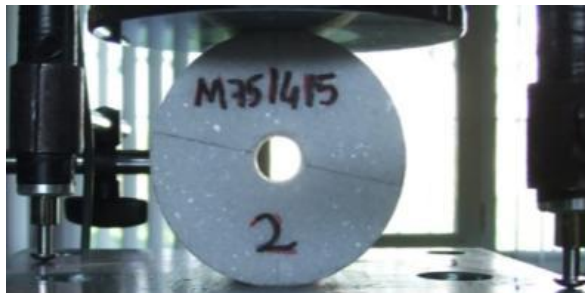
Figure 8. 25 MR specimen while loading
