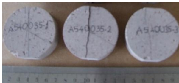
Figure 8. 21 FBD specimens after fracturing
