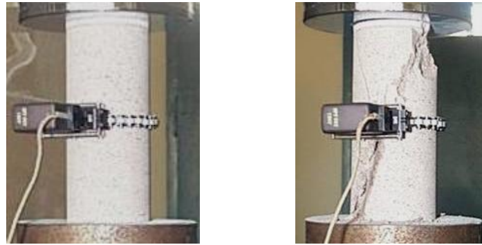
Figure 8. 1 UCS test specimen with circumferential extensometer before and after the test
