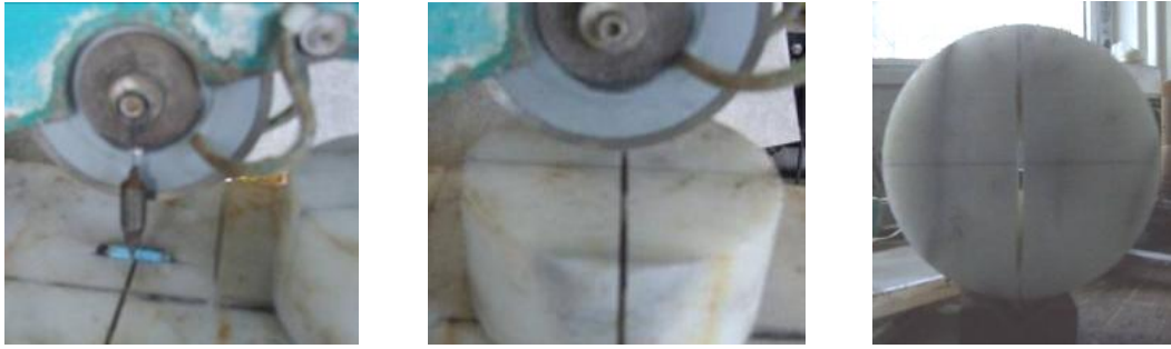
Figure 8. 12 Plum-line and flat iron stick adjustment for the second notch (on the left), specimen placement (at the center) and prepared specimen (on the right)
