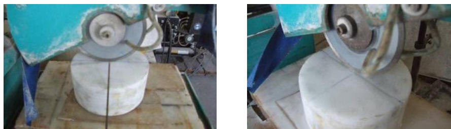
Figure 8. 11 Specimen placed exact location before cutting (on the left) and after cutting (on the right)
