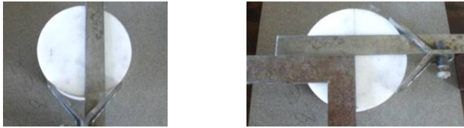
Figure 8. 8 Diametral line drawing with goniometer (on the left) and line perpendicular to diametral line drawing with goniometer and set-square (on the right)
