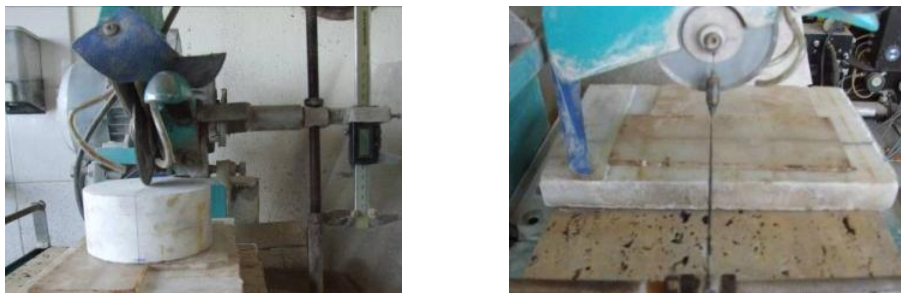
Figure 8. 10 Digital caliper adjustment (on the left) and plum-line and flat iron stick adjustment (on the right)
