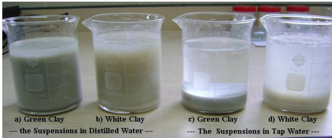
Figure 21. Sedimentation Behavior of the Suspensions (3% Clay; After 24 Hours)
