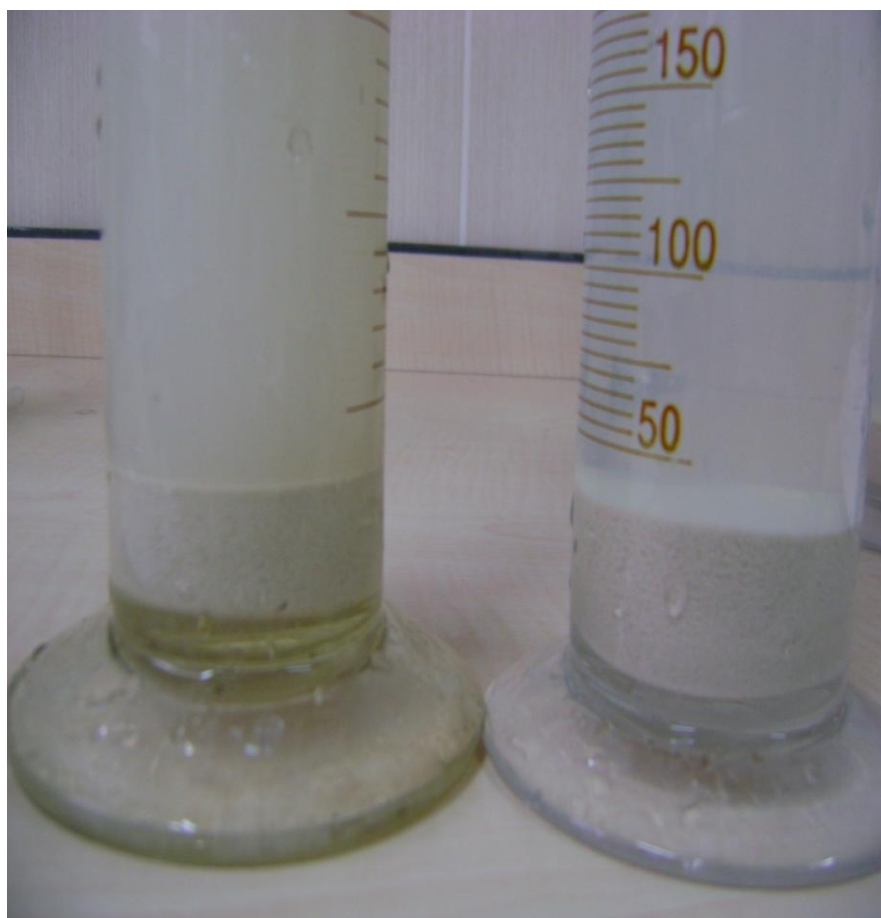
Figure 32. The White Clay Floes at Calcium Concentration: 100 mg / L on the left side and 500 mg / L on the right side (3% Borax; 3% Clay; 100 ml-UMA Magnafloc as flocculant; pH=9.40)
