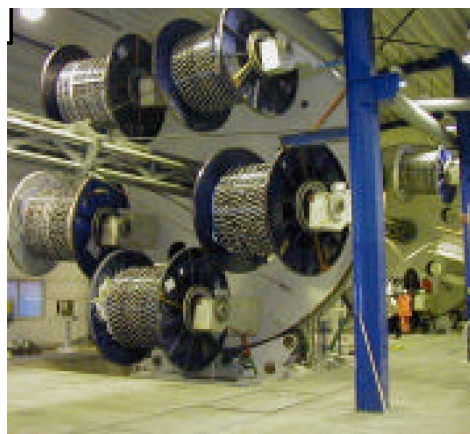
Figure 1.9 Carbon fiber rods are wound helically around these very long tendons. 3
