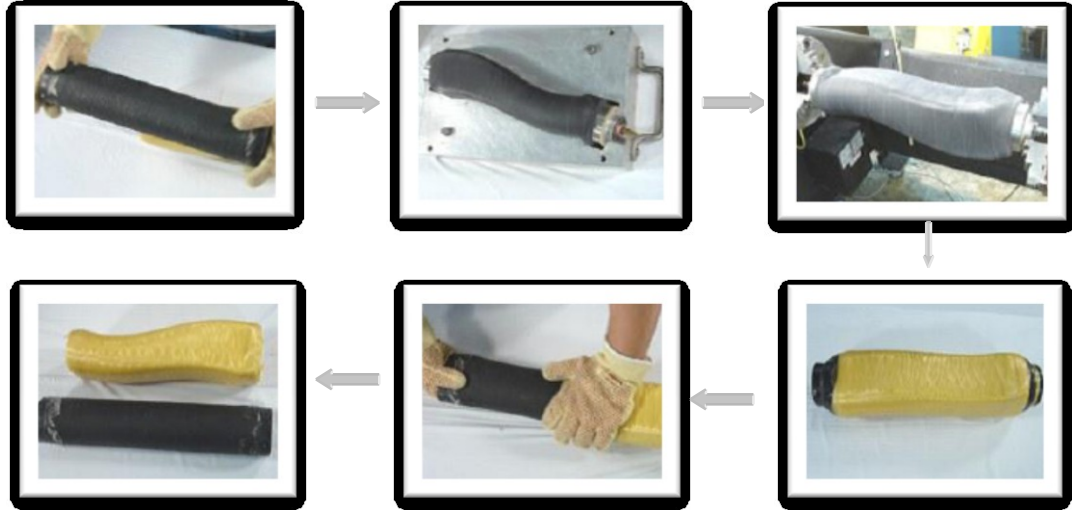
Figure 1.13 Reusable mandrels with shape memory polymers [16]
