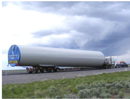
Figure 1.11 Transport of a segment of wind turbine tower. 5
