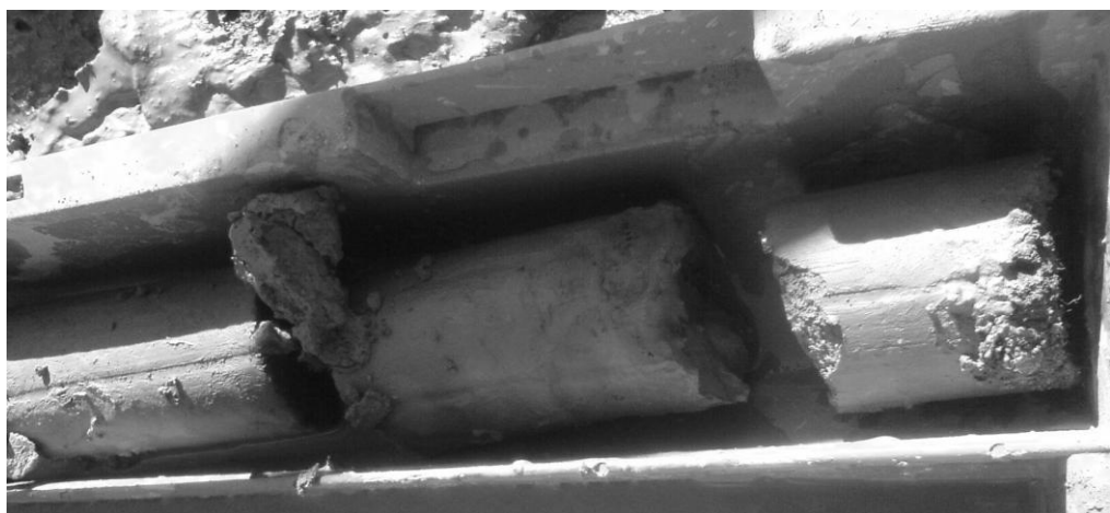
Figure 2.9 Recovered core-barrel sample.
