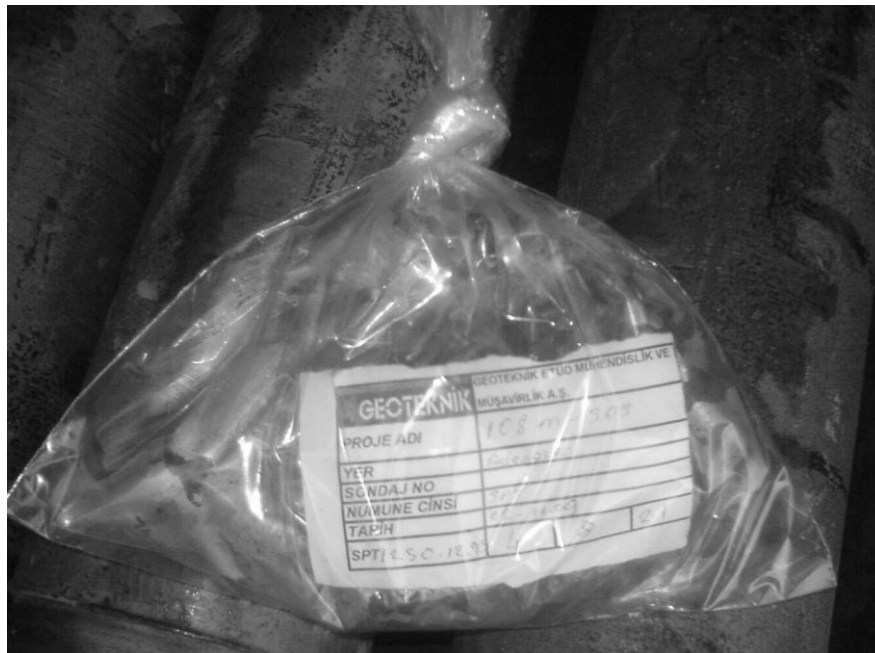
Figure 2.6 Disturbed sample recovered during SPT.
