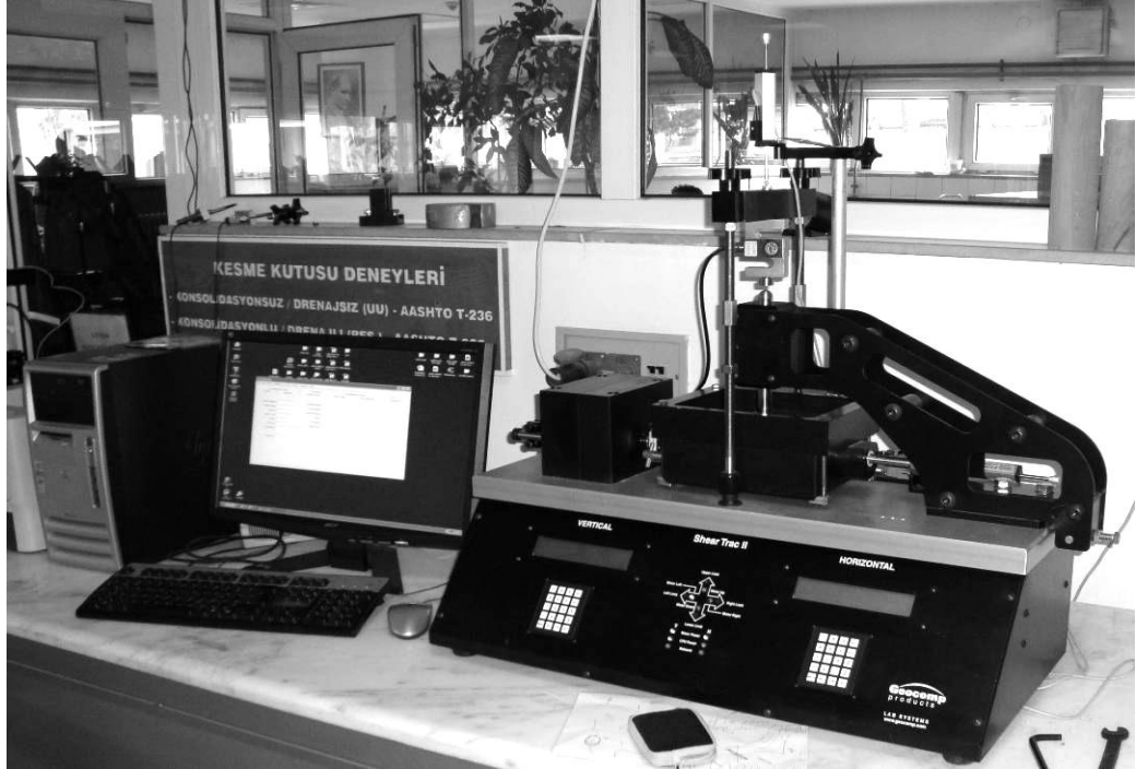
Figure 3.3 ShearTrac II, the cyclic direct simple shear apparatus used for the tests.
