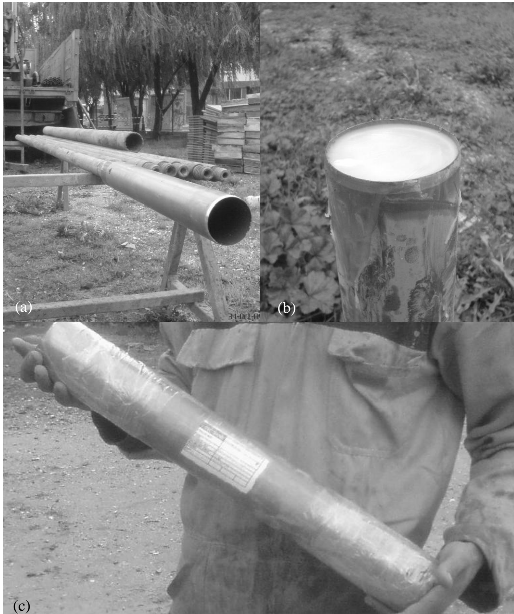
Figure 2.4 Preparation of an undisturbed sample for shipment: a) Thin-Walled Tube sampler is mounted to drilling rod, b) upper end of a Thin-Walled Tube sampler is sealed with wax, c) Sealed and identified thin-walled tube sample is ready for shipment.
