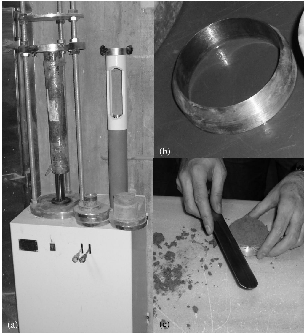
Figure 3.5 Lab equipment used for specimen recovery: a) Shelby tube installed on an electro-hydraulic jack, b) specially manufactured small rings, c) knife trimming the specimen.
