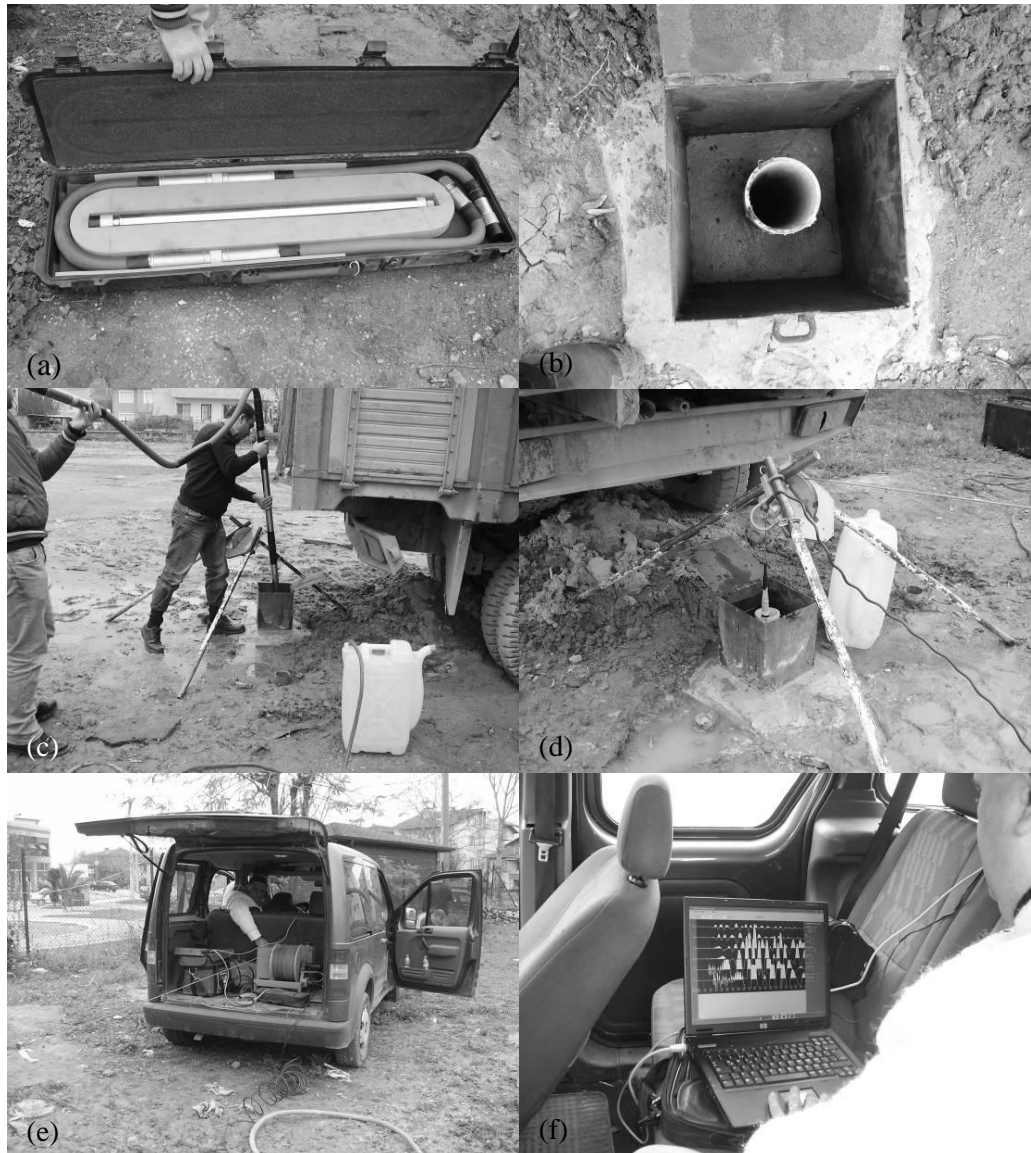
Figure 2.12 The equipment and stages of P-S suspension logging in Adapazarı: a) the probe, b) the borehole with PVC pipe, c) lowering the probe inside the borehole, d) suspending the probe inside the borehole with a cable, e) the winch unit, and f) laptop used for recording and analyzing data.
