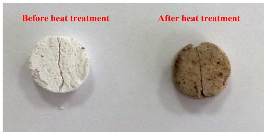
**Figure 5.4** Optical images of the PCL-coated HAp pellets before (left) and after (right) the heat treatment process at 200 °C. Color and mass change was observed on the heat treated sample.
