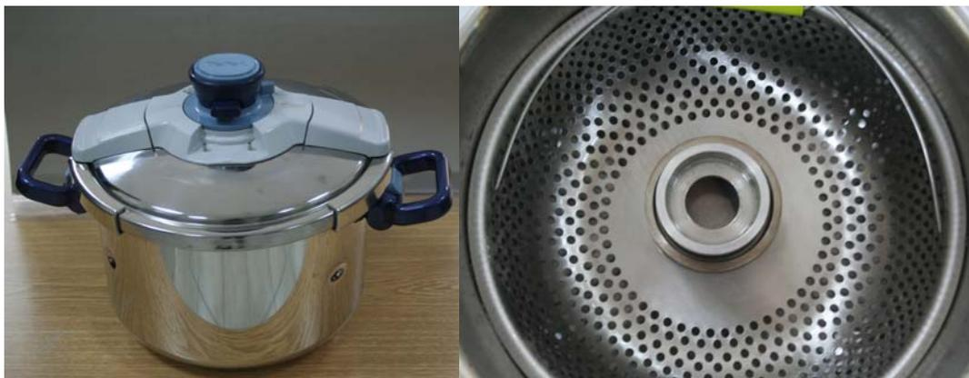
**Figure 2.1** A view of pressure vessel used in high pressure experiments. (left: general view, right: interior part showing the modification). This modification was done to put more water inside. Additionally, it has made the sample container stationary and disabled the opportunity of sample spilling into the vessel.
