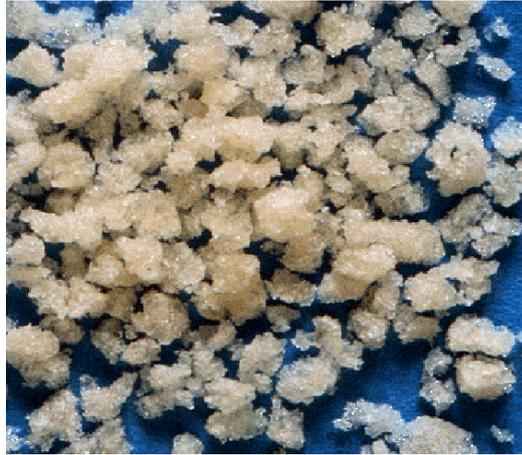
**Figure 1.4** An optical image of Immix Extenders (Osteobiologics, Inc.), a particulate form of poly(lactic-co-glycolic) acid (abbreviated as PLGA) [16]
