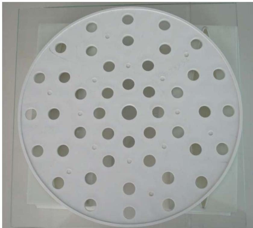
**Figure 2.7** The mold used to produce disc shaped bulk gypsum samples
