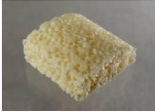
**Figure 1.3** An optical image of porous alumina ceramic [12]
