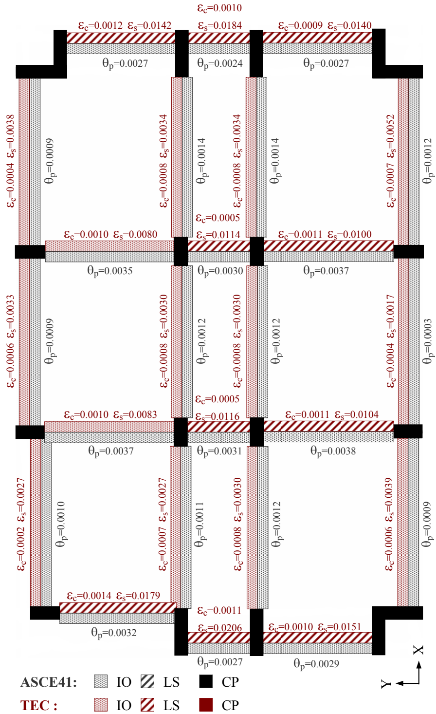
Figure C.5 Comparative assessment of the first floor beams in the Bingöl building as per ASCE/SEI-41 and TEC
