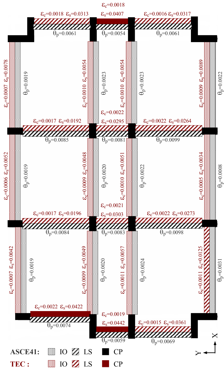
Figure 5.18. Comparative assessment of the ground floor beams in the Erzincan building as per ASCE/SEI-41 and TEC
