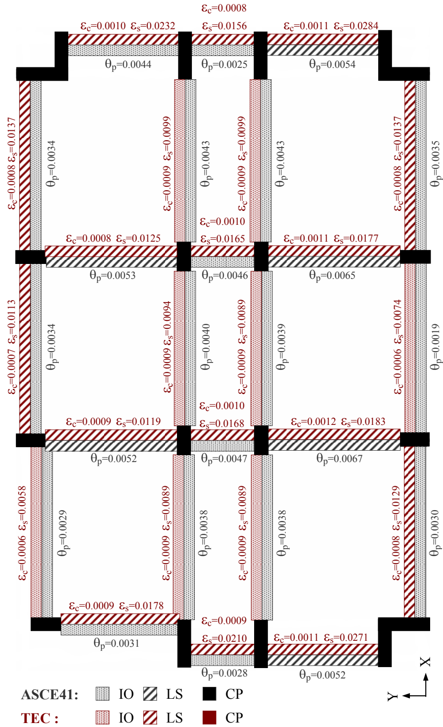
Figure C.4 Comparative assessment of the second floor beams in the Bolu building as per ASCE/SEI-41 and TEC
