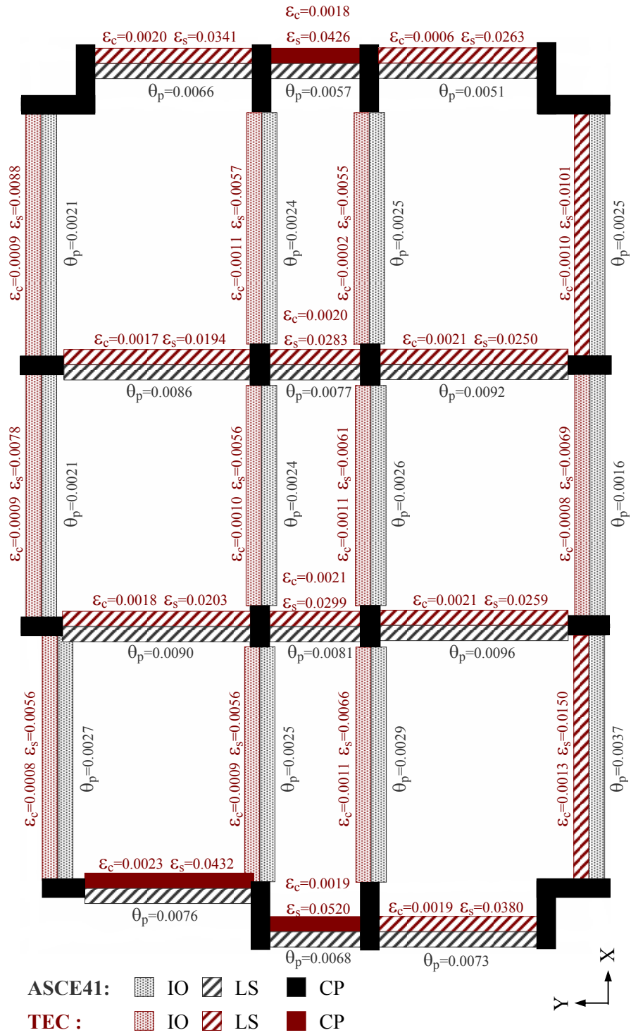
Figure C.1 Comparative assessment of the first floor beams in the Erzincan building as per ASCE/SEI-41 and TEC
