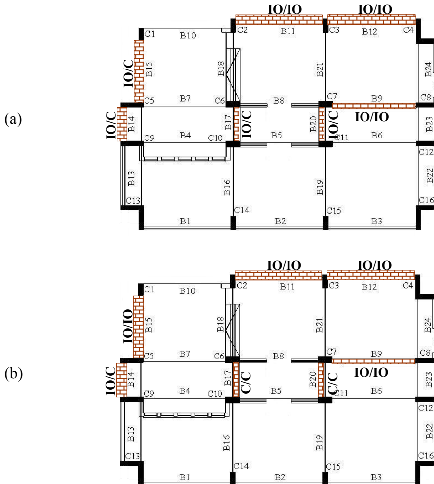
Figure 5.21. Comparison of the observed and calculated damage of the ground story infill walls regarding the (a) Erzincan and (b) Bolu buildings. (Observed Damage/Calculated Damage) IO : Immediate Occupancy C: Collapse
