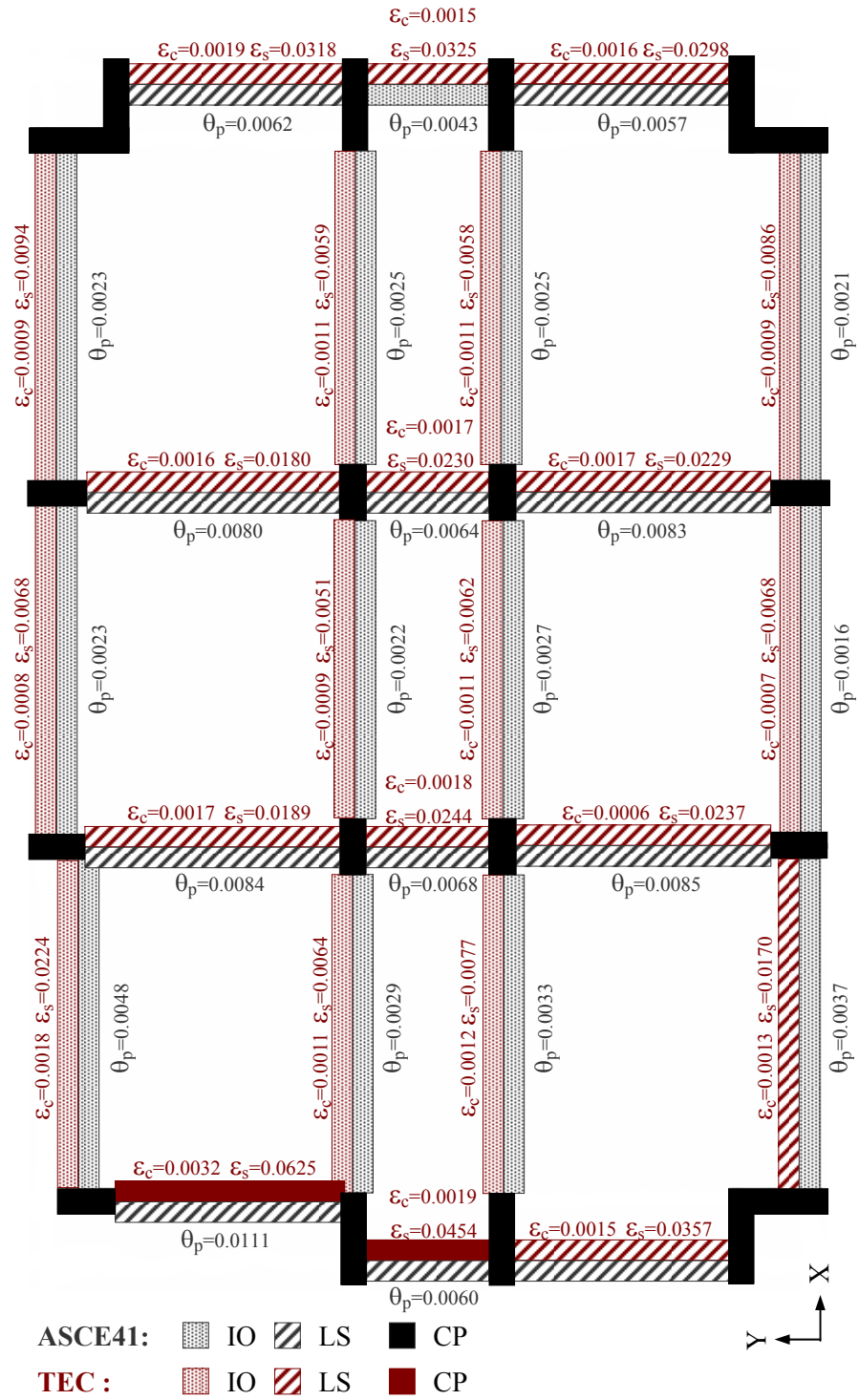
Figure C.2 Comparative assessment of the second floor beams in the Erzincan building as per ASCE/SEI-41 and TEC
