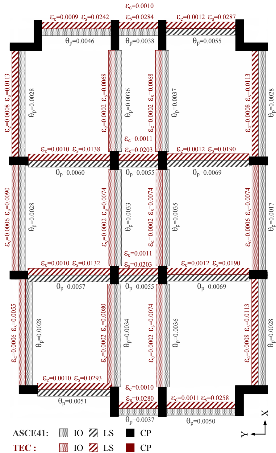
Figure 5.19. Comparative assessment of the ground floor beams in the Bolu building as per ASCE/SEI-41 and TEC
