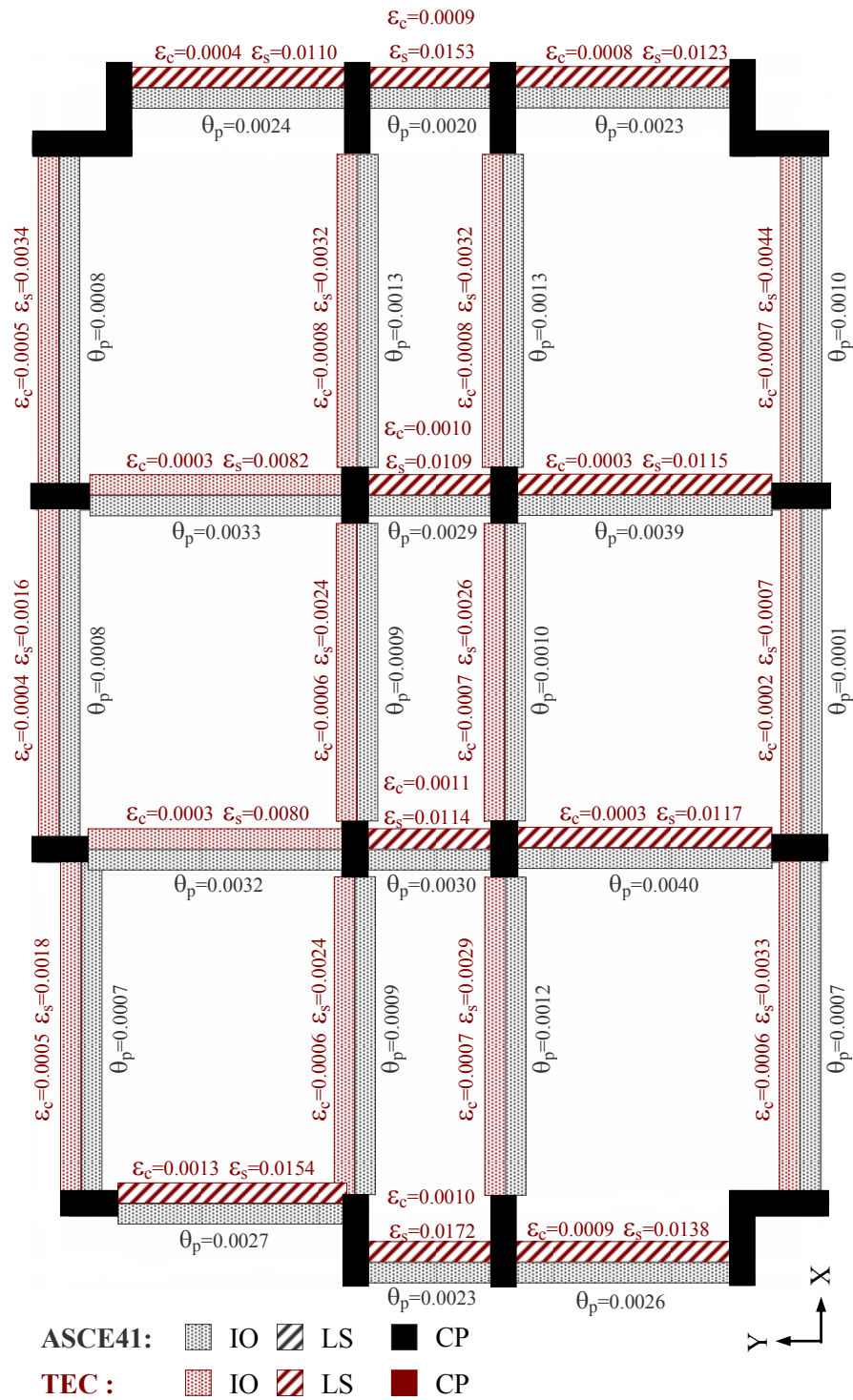
Figure 5.20. Comparative assessment of the ground floor beams in the Bingöl building as per ASCE/SEI-41 and TEC
