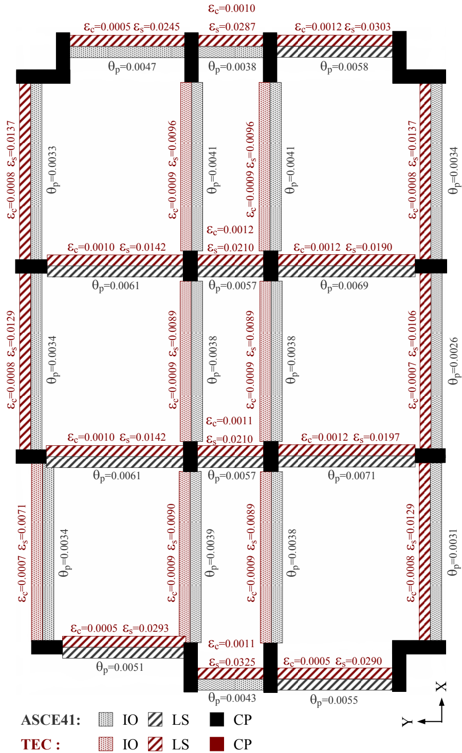
Figure C.3 Comparative assessment of the first floor beams in the Bolu building as per ASCE/SEI-41 and TEC
