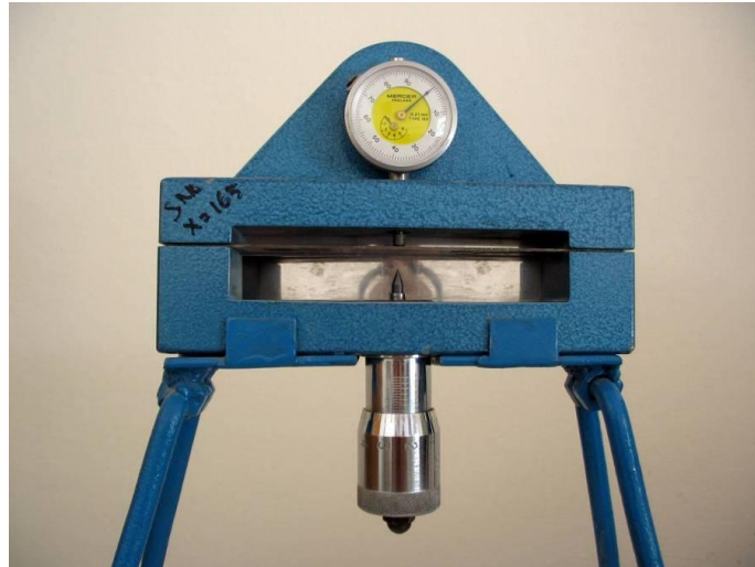
Figure 3.1. NCB Cone Indenter
