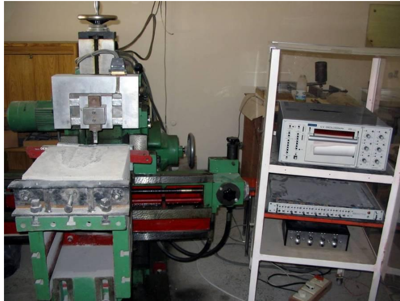
Figure 3.4. Rock Cutting Setup
