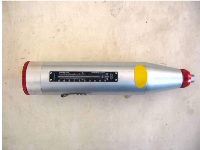
Figure 3.3. L-Type Schmidt Hammer
