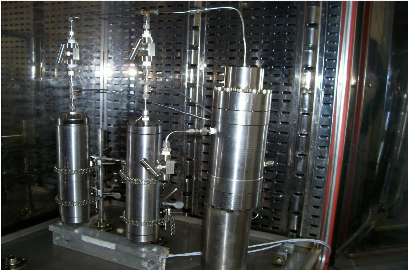
Figure C. 1 Mixing cylinder and core holders inside the oven
