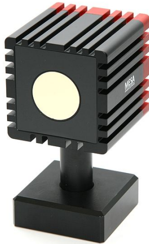
Figure 3.2: SwissRanger SR4000 time-of-flight range camera.
