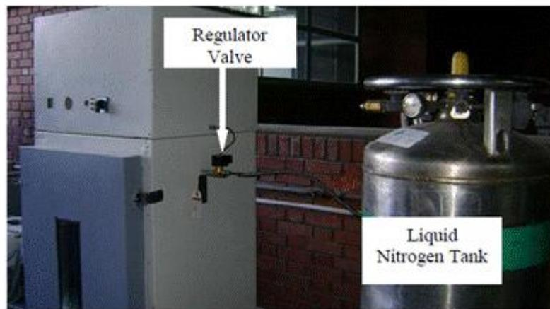
**Figure 3.5- Liquid nitrogen supply arrangements**
