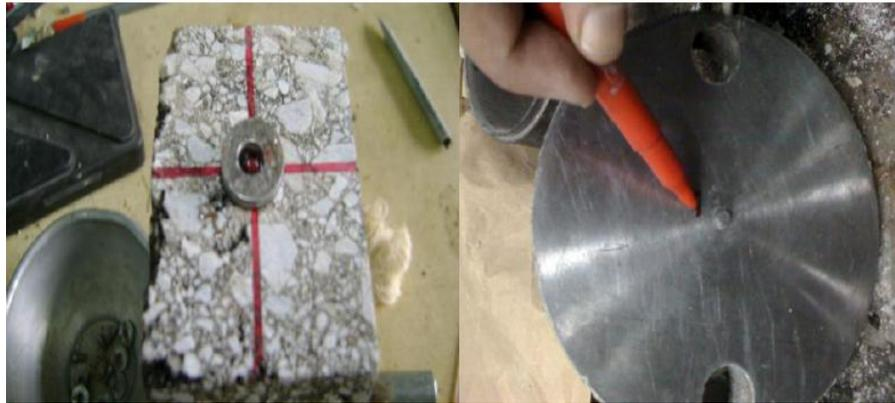
**Figure 3.19- Centring of test specimen by gluing the ring and fixing to the projection**
