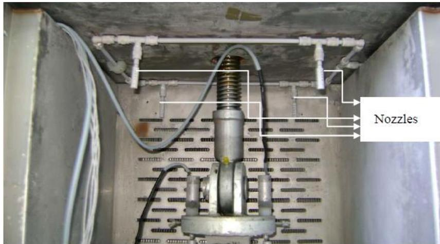
**Figure 3.7- Nozzle system placed in the device**
