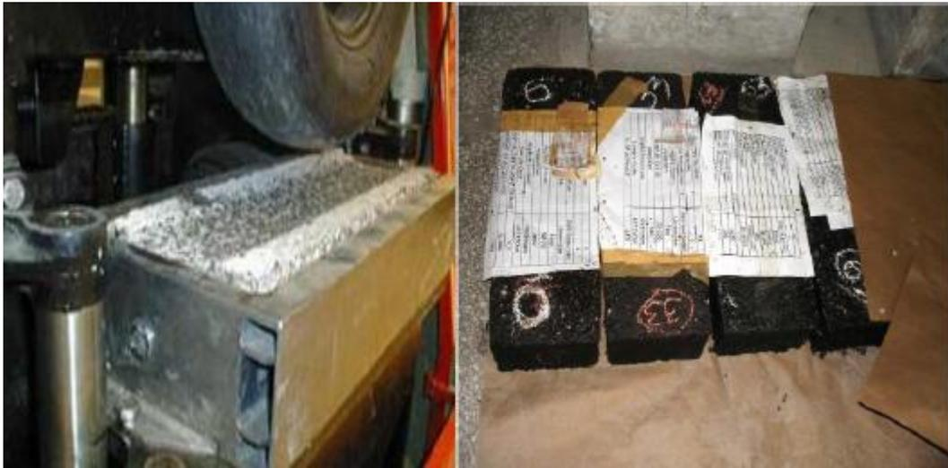
**Figure 3.16- Slab sample preparation during and after compaction**
