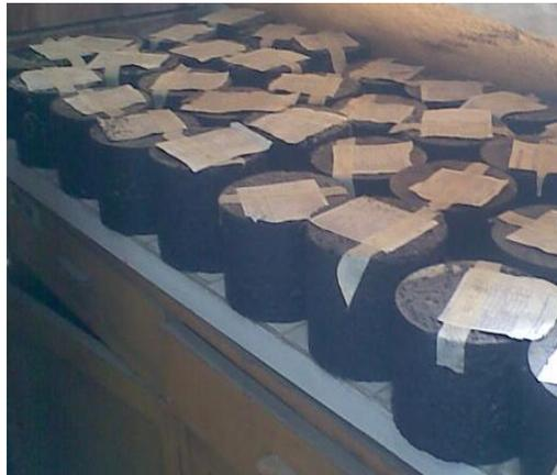
**Figure 3.15- Mix design samples according to the Superpave method**
