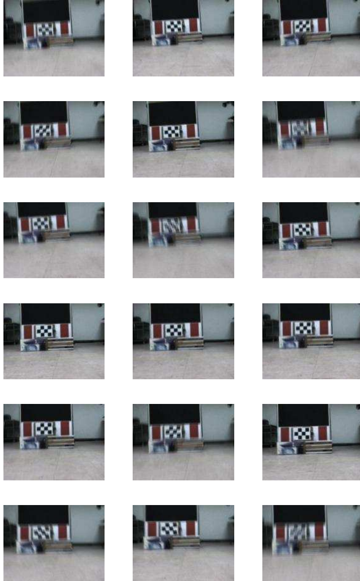
Figure A.7: 725 to 742 frames of the test video recorded while our experimental robotic platform RHex was walking with 0.8 velocity coefficient.
