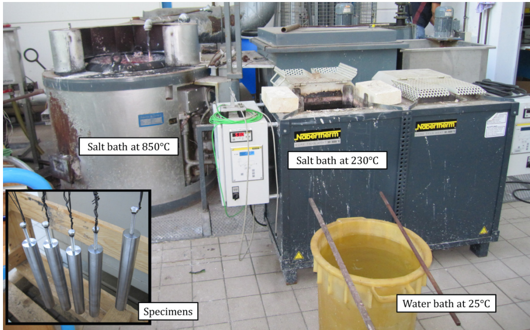
Figure 17: Salt bath quenching set up
