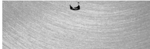
Figure 24 Unmelted part observed on the cross section of the sample
