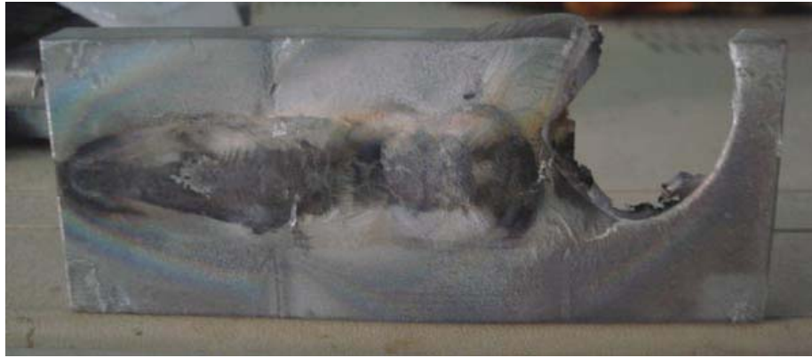
Figure 22 Excessive heat caused melting of the specimen
