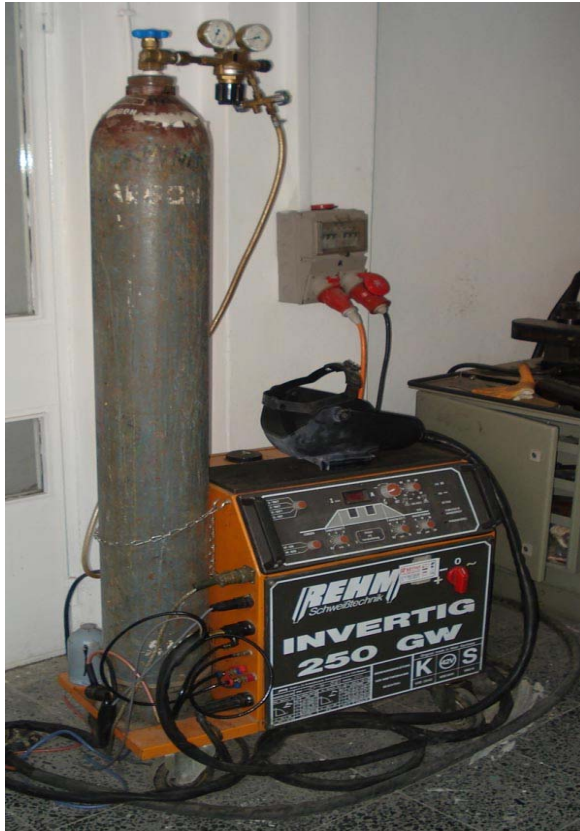
Figure 17 Power Source of the MVT Equipment
