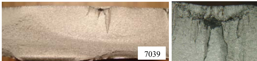
Figure 60 Macro-photos of the fatigue fractured surface of 7039 aluminum alloy.
