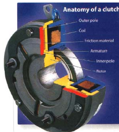
Figure 4.15: Anatomy of an Electromagnetic Brake [84]
