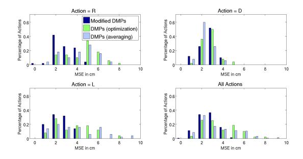
Figure 5.8: Comparison of the DMPs and the modified DMPs using the test set. Histogram of the MSEs are shown which are divided into bins of size 1 cm.
