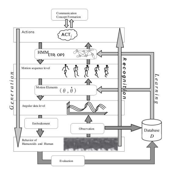
Figure 2.2: Overall architecture of the mimesis model. Figure taken from [1] with the kind permission of the corresponding author.
