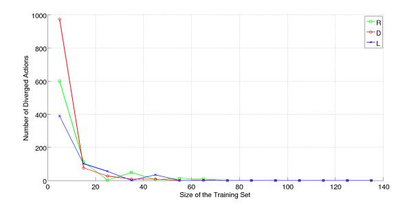
Figure 5.4: Number of diverged actions vs. training set size. For each action 1000 random starting points are used to test convergence where a generated action is considered as diverged if end-effector's distance to the goal is higher than 5cm after an execution of 1.5 seconds.
