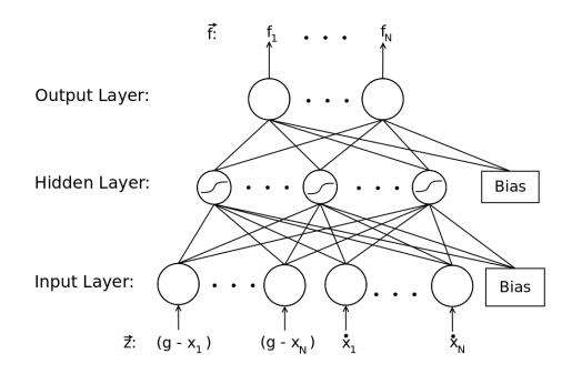
Figure 3.4: Feed forward neural network used as the non-linear part of the modified DMPs.
