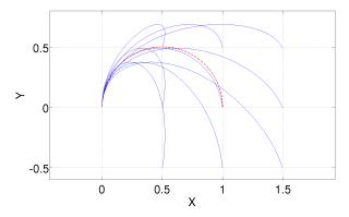
(a) Goal adaptation of DMPs for simulated data. The red dashed curve is the demonstrated trajectory and the blue curves are the trajectories generated by DMPs.
