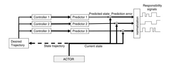
Figure 2.5: MOSAIC in learning/recognition mode. Observed trajectory is treated as the desired trajectory and the resulting responsibility signals are stored as the parameters of observed action for learning. For recognition, responsibility signals can be compared with the ones in the repertoire. Figure taken from [2] with the kind permission of the corresponding author.
