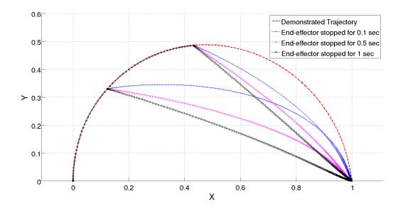
Figure 3.2: Effects of stopping the end-effector for different durations on the generated trajectory.
