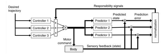
Figure 2.4: MOSAIC in control mode. Generated motor command is the weighted sum of the outputs of controllers where these weights are calculated according to the prediction errors. Figure taken from [2] with the kind permission of the corresponding author.
