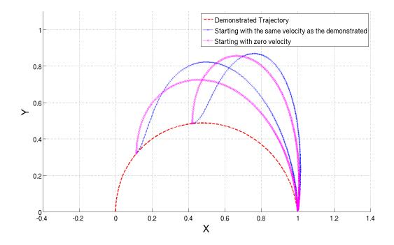
Figure 3.3: Different trajectories generated by taking different points on the demonstrated trajectory as starting points.
