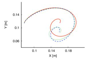
(b) Goal adaptation of DMPs for a human demonstration. The red curve is the demonstrated trajectory, blue dashed curve is the trajectory of the human for the new goal and the green dotted curve is the one generated by DMPs. Figure taken from [10] with the kind permission of the corresponding author.
