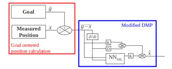
Figure 3.5: Overall architecture of the modified DMPs.  $NN_{SEL}$  is the neural network of the selected action.
