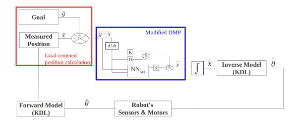
Figure 5.11: Action generation architecture implemented on the iCub platform.  $NN_{SEL}$  is the neural network of the selected action and  $\dot{\bar{\theta}}$  (joint velocities) is sent to the actuators as motor commands.
