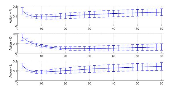
Figure 5.3: Results of the optimization procedure for K values. X axis is the tested K values and Y axis is the average work required from the non-linear part for one sample of a trajectory. Optimized K values are 10, 26 and 10 for R, D and L respectively.
