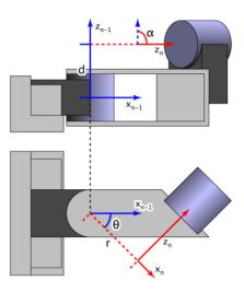
Figure B.2: Example of D-H parameters between two joints. Figure taken from [4].
