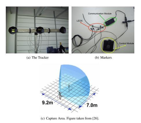
Figure 4.2: The Components and the Capture Area of the Motion Capture System
