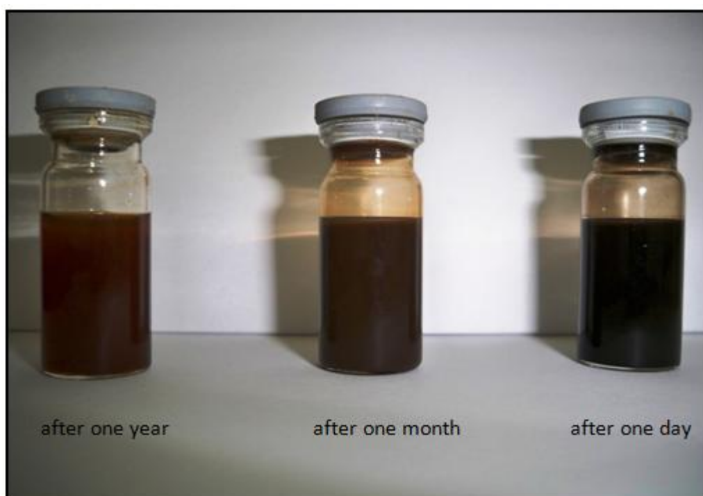
Figure 25. Pictures of the magnetite nanoparticle solutions taken at different times after the synthesis.
