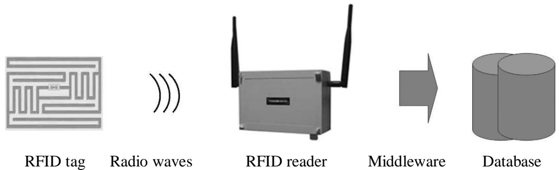
Figure A.1: The basic elements of RFID technology are tags, readers, and middleware (Langer et al., 2007)
