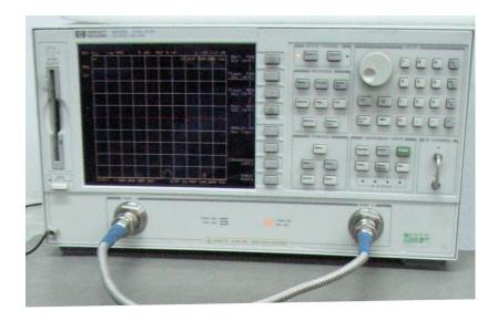
Figure 4.6: Agilent 8720D vector network analyzer
