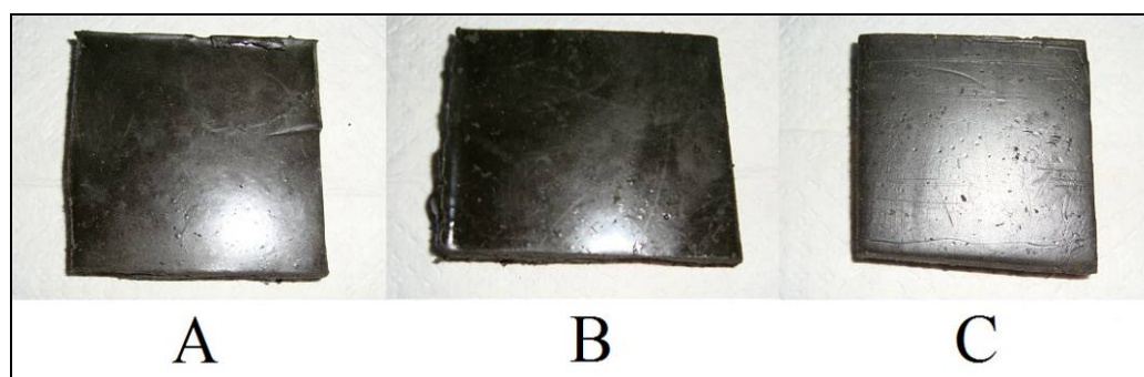
Figure 4.15 XLDB-3 Aged for 120 days at (A) 45°C, (B) 55°C and (C) 65°C
