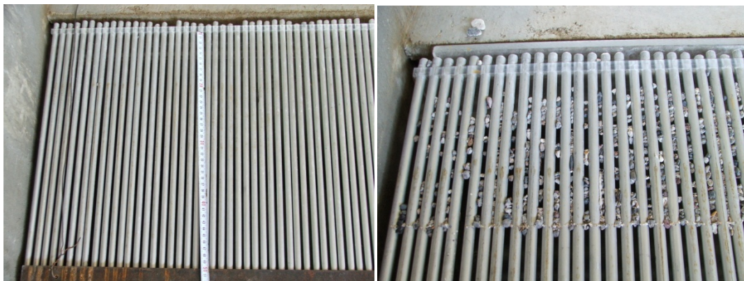
Figure 3.6 Tyrolean screen with e_1 = 3 mm clear distance between bars (clean and clogged after the experiment)
