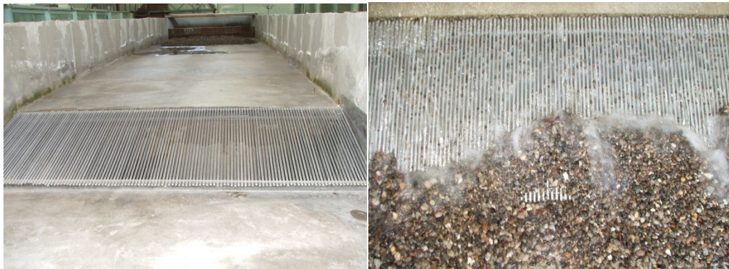
Figure 3.7 Tyrolean screen with e_2 = 6 mm clear distance between bars (clean and clogged during the experiment)
