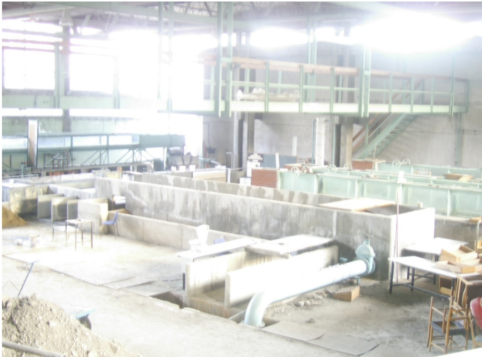
Figure 3.2 General view of the Tyrolean weir model
