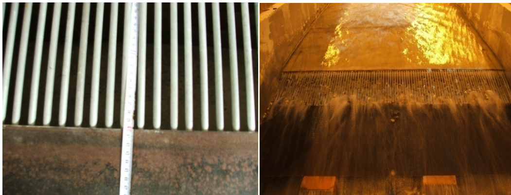
Figure 3.8 Tyrolean screen with e_3 = 10 mm clear distance between bars (clean and clogged during the experiment)
