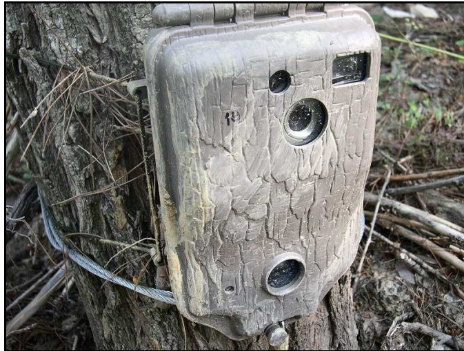
Figure 2-4. A picture of DeerCam DC300 camera trap. The muddy appearance was result of wild boar rubbing.
