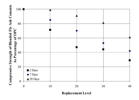
Figure 4.6 Strengths of Blended Fly Ash Cements as Percentage of that of OPC
