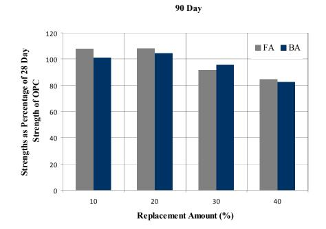
Figure 4.11 Compressive Strengths of Blended Cements at 90<sup>th</sup> Day as Percentage of Strength of OPC at 28<sup>th</sup> Day
