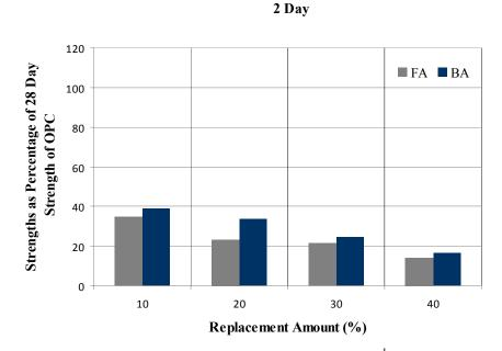
Figure 4.8 Compressive Strengths of Blended Cements at 2<sup>nd</sup> Day as Percentage of Strength of OPC at 28<sup>th</sup> Day
