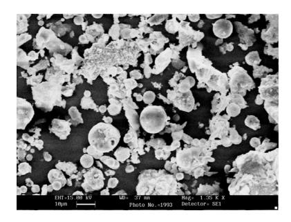
Figure 4.2 Microstructure of Fly Ash
