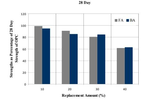
Figure 4.10 Compressive Strengths of Blended Cements at 28<sup>th</sup> Day as Percentage of Strength of OPC at 28<sup>th</sup> Day
