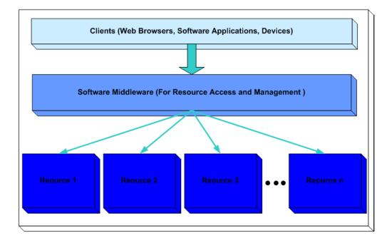
Figure 1.1: Distributed System Stack
