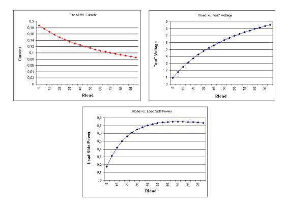
Figure 2.2: Rload vs. Current, Voltage, and Power
