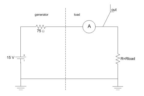
Figure 2.1: A Direct Current Electrical Circuit
