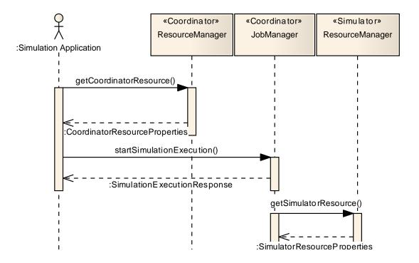
Figure 2.4: Initialization Stage of Sim-PETEK Workflow
