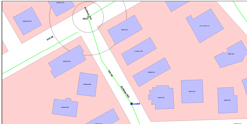
Figure 6.64 Position of leak 8 and the nearby valve with its effective area
