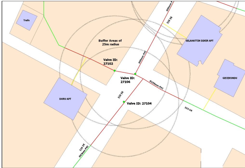
Figure 6.21 Noise Data Loggers with Serial Numbers 3606 and 3622 Placed On Valves #27102 and #27104 and Their Corresponding Effective Areas
