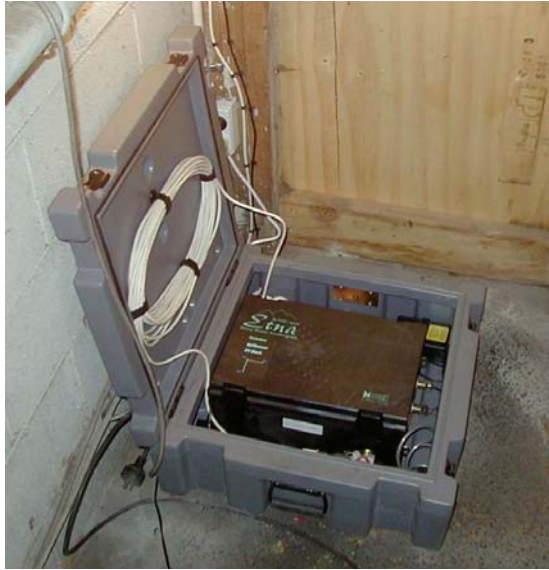
Figure 5: An accelerograph ( www.geonet.org.nz )
