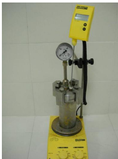
Figure 3.1 Laboratory made stainless steel autoclave used in hydrothermal treatments.
