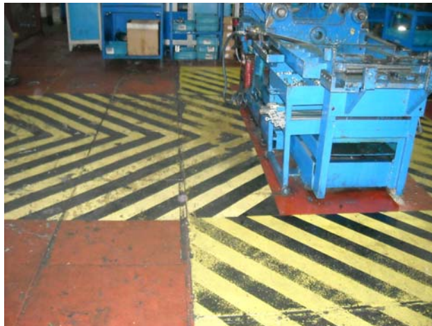
Figure A.1: The yellow-black markings on the floor draw the attention of the workers
