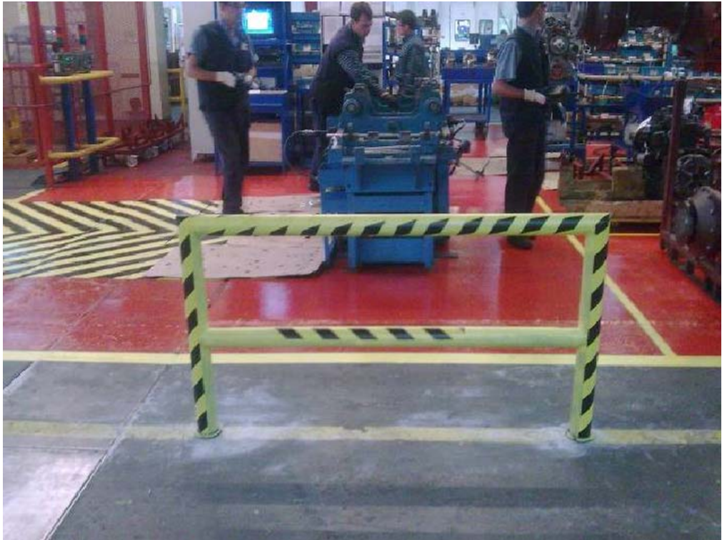
Figure A.2: The barrier in front of the working area in order to avoid the risk of a forklift crash to the operator.
