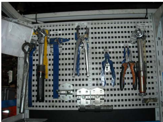
Figure A.3: The instruments put in order by application tool of WCM, 5S.
