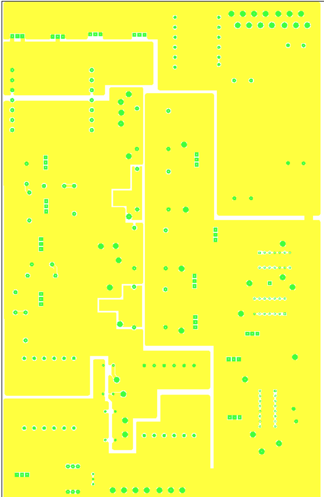
Fig.B.2 Bottom side layout of Z-source full bridge dc/dc converter
