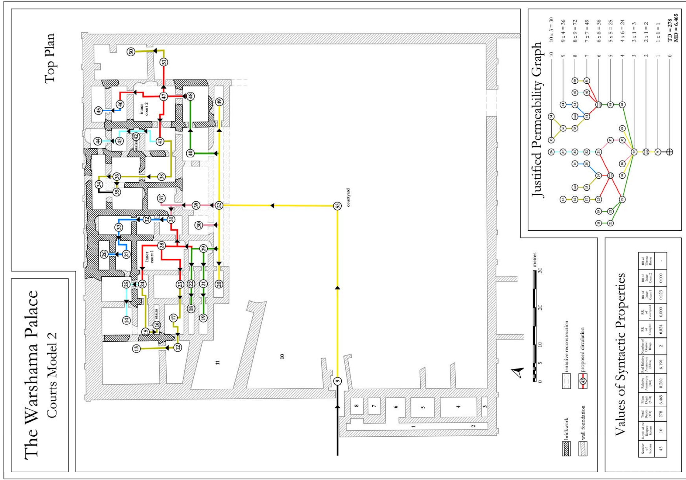
APPENDIX F: Composite plan of the Warshama Palace based on Courts Model 2, showing the color coded plan, the justified permeability graph and the table of syntactic properties.
