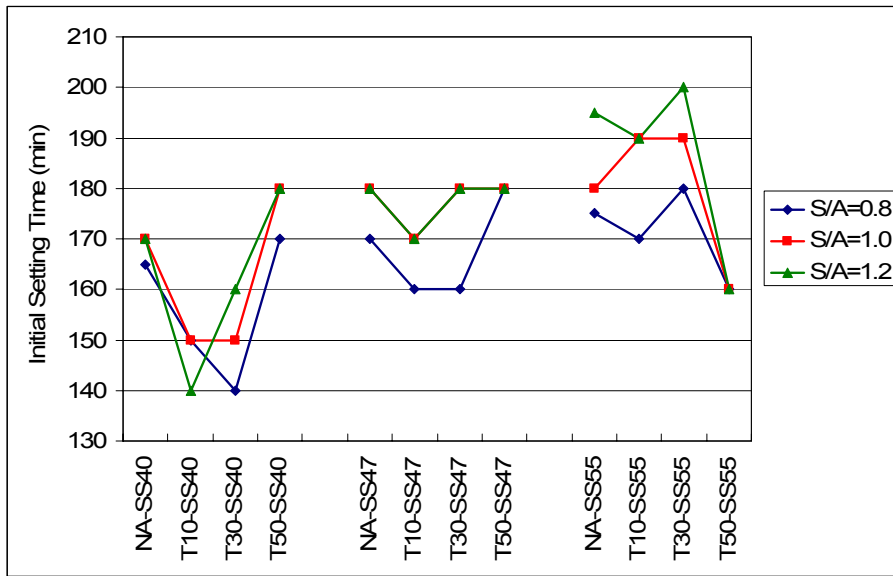
Figure 4.5 Initial setting times of the samples containing trass additive
