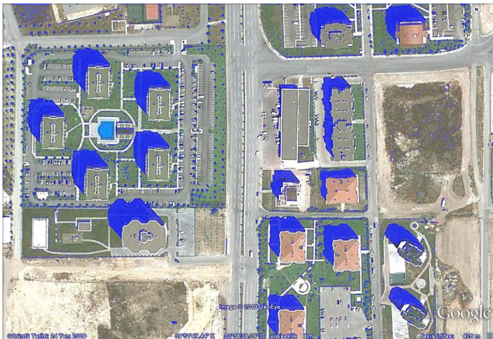
Figure 56 – NSVDI with auto threshold [4] combined with removal step of bluish and greenish regions [36]
