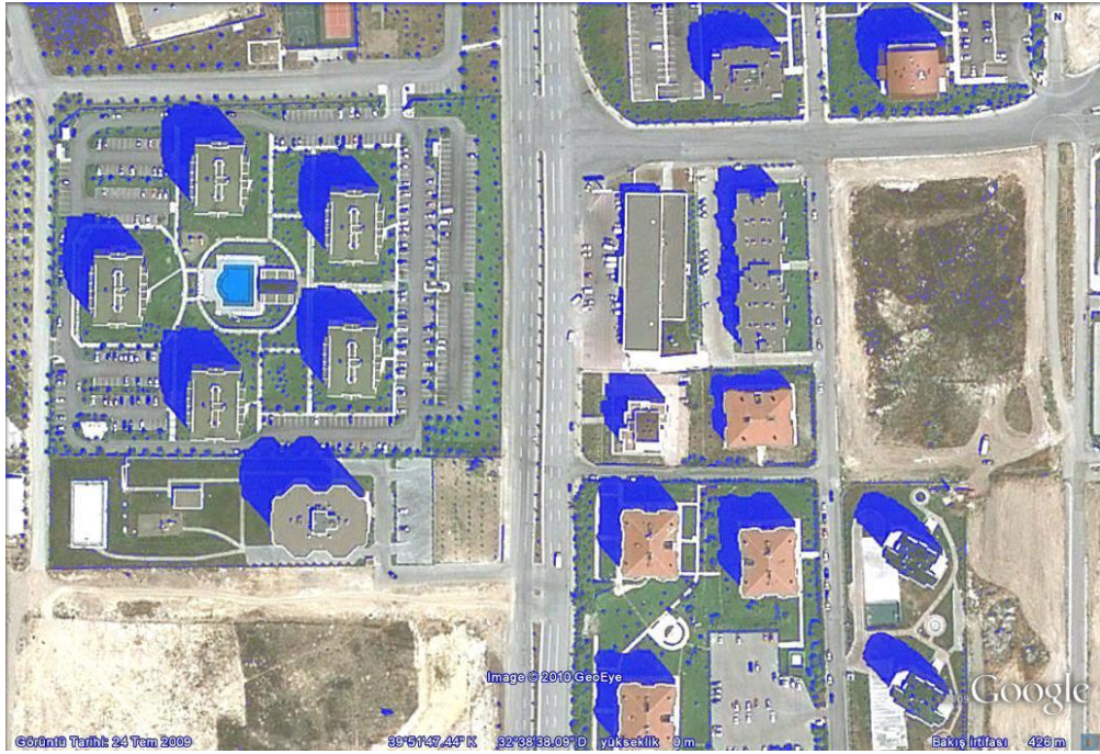
Figure 63 – (H_e+1) / (I_e+1) ratio auto threshold method [34] combined with removal of bluish and greenish regions [36]
