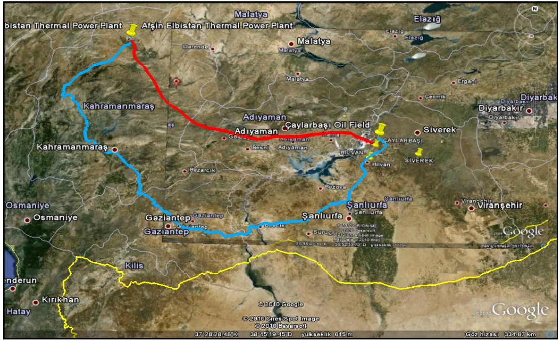
Figure 5.7: Comparative Satellite Display of Pipeline Route and Tanker Route Between Afşin Elbistan Power Plant and Çaylarbaşı Oil Field
