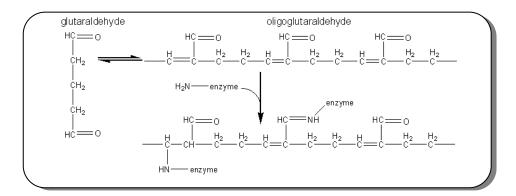
Figure 21: Coupling of glutaraldehyde with enzyme
