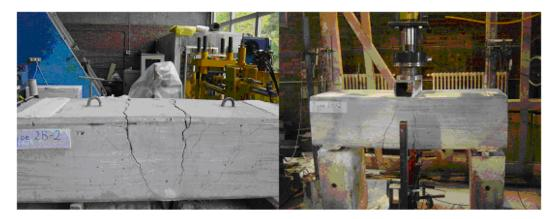
Figure 4.28 Type 2B-2 Specimen after Static Loading Test
