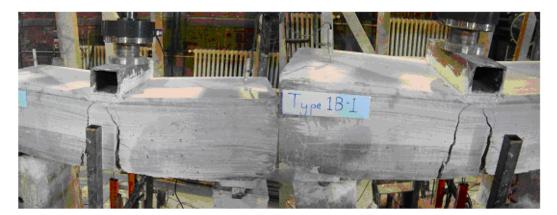
Figure 4.22 Type 1B-1 Specimen after Static Loading Test
