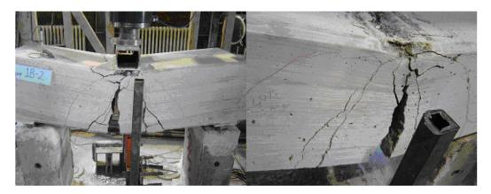
Figure 4.24 Type 1B-2 Specimen after Static Loading Test
