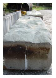
Figure 4.5 Concrete Face After Fire Test (Type 1B-1)
