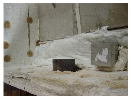
Figure 4.2 Placement of the Cube Specimen into Furnace
