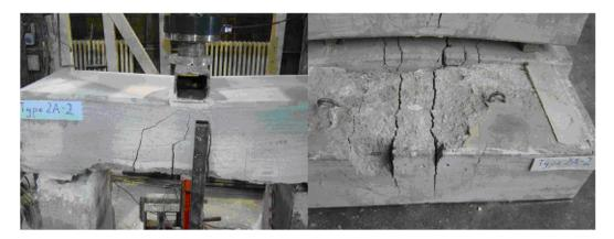
Figure 4.18 Type 2A-1 Specimen after Static Loading Test
