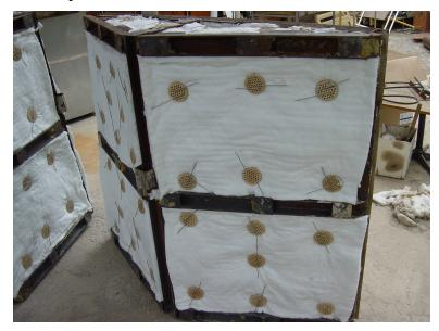
Figure 3.10 Ceramic Fiber Isolation on the Furnace Flap
