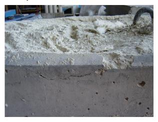
Figure 4.8 Concrete Face After Fire Test (Type 1A-1)
