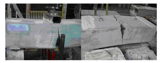
Figure 4.16 Type 1A-2 Specimen after Static Loading Test
