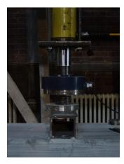
Figure 3.14 Load Cell
