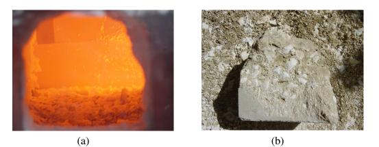
Figure 4.11 (a) Concrete Face in Fire Test, (b) Cube Specimen after Fire Test
