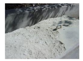
Figure 4.6 Concrete Face After Fire Test (Type 2A-1)
