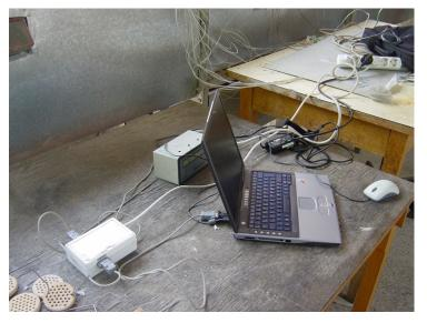
Figure 3.11 Data Acquisition System
