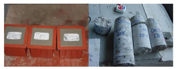
Figure 3.16 Compression Test Samples
