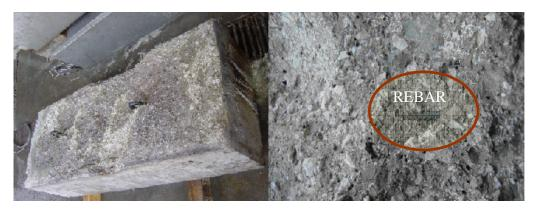
Figure 4.9 Concrete Faces after Fire Test (Type 2B-1)
