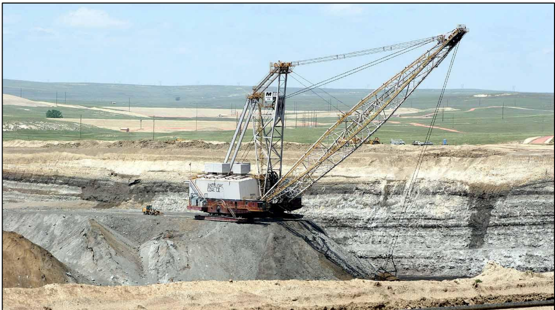
Figure 2.1 Dragline Stripping in a Coal Mine (Anonymous, 2008)
