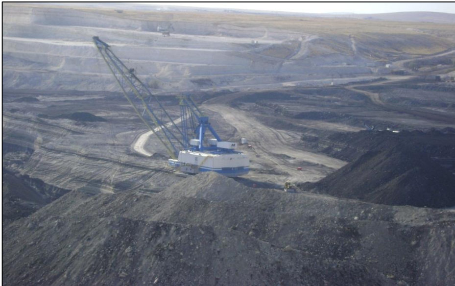
Figure 1.1 Dragline Operation in DemirExport Coal Mine
