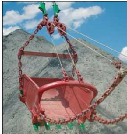
Figure 3.2 Bucket and Rigging Mechanism in the Operation (Esco Dragline Buckets, 2010)
