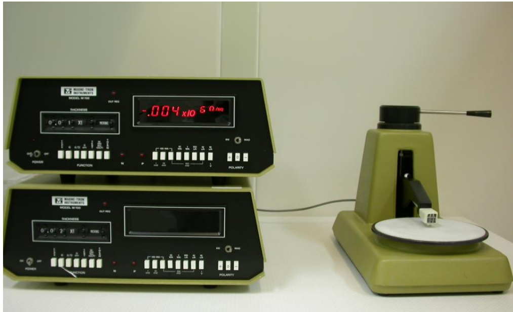
Figure 2.3: Four-point probe used in the sheet resistance measurements of the vanadium sputtered sample.
