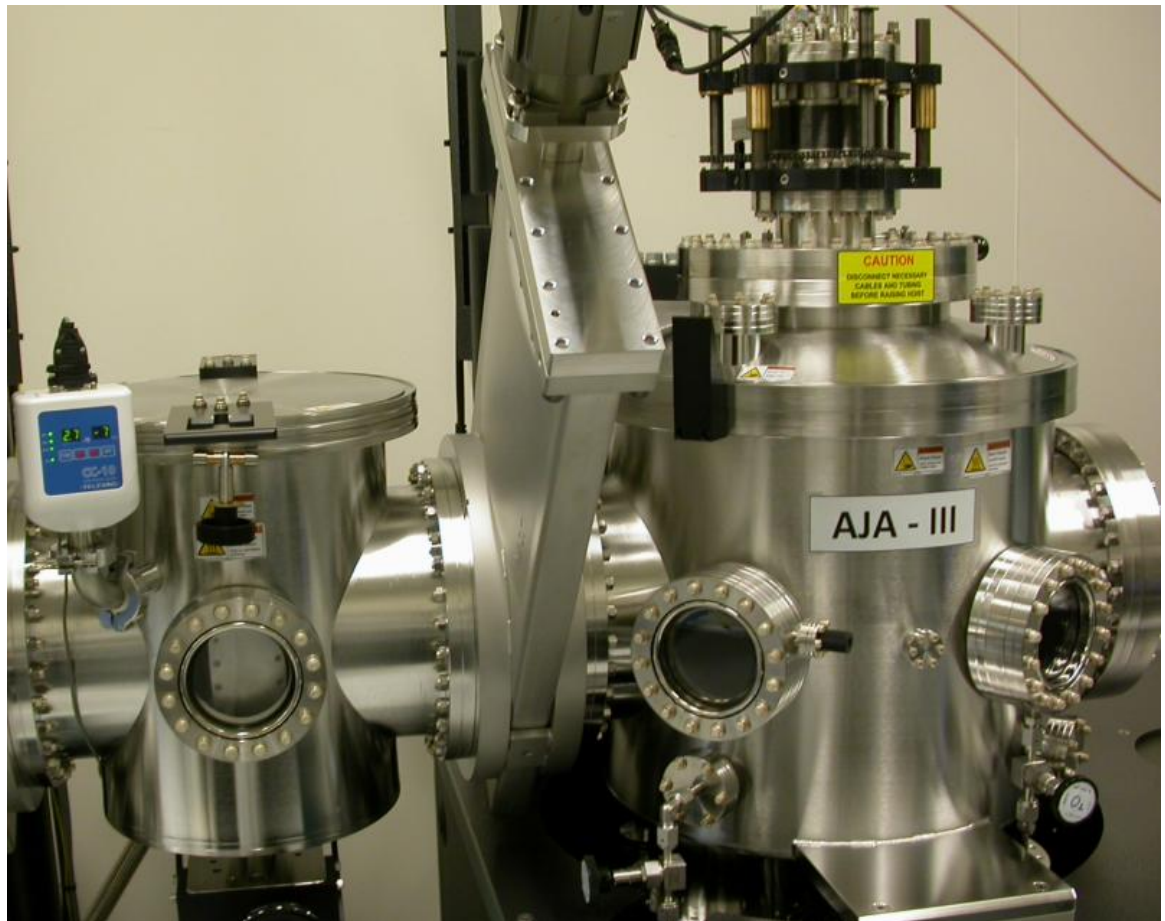
Figure 2.1: The sputtering system used in the vanadium oxide depositions in METU MEMS Center.
