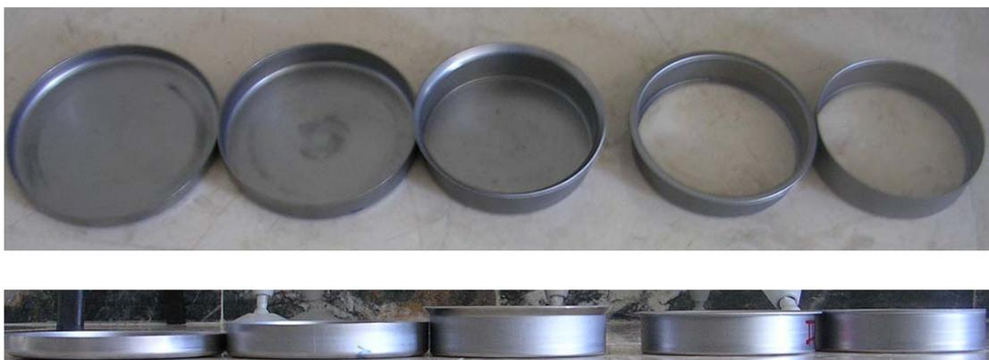
**Figure 5.17:** Deep Drawing stages and the final sample
