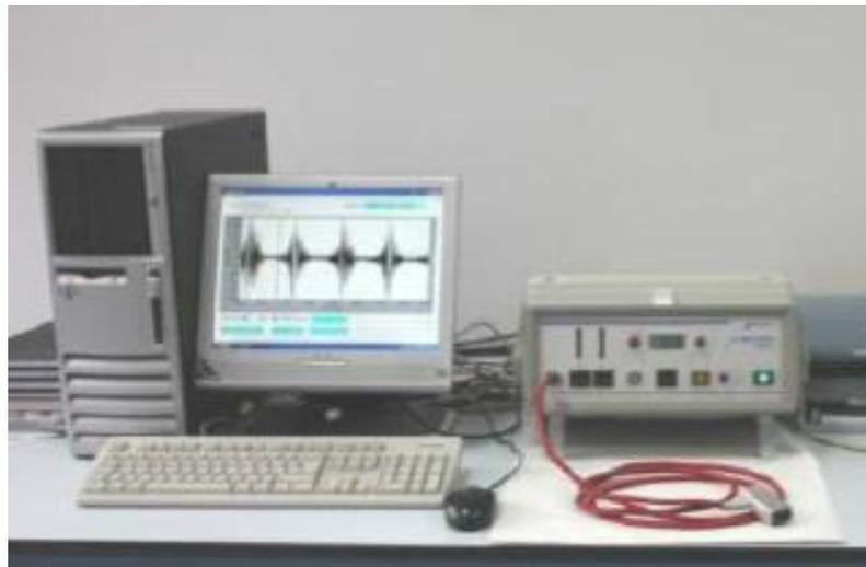
**Figure 4.13:** Stresstech Rollscan- $\mu$ Scan 500-2 device Magnetic Barkhausen Noise Equipment
