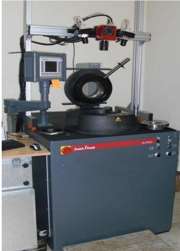
**Figure 4.4:** BUP 600 hydraulic press with GOM ARAMIS
