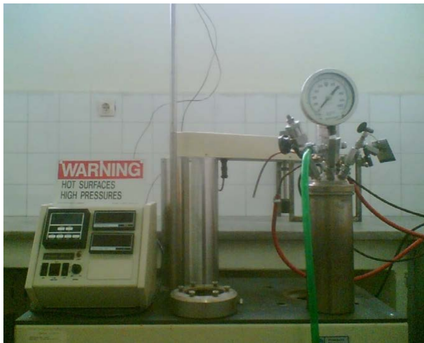
Figure 3.5 Titanium autoclave and its parts
