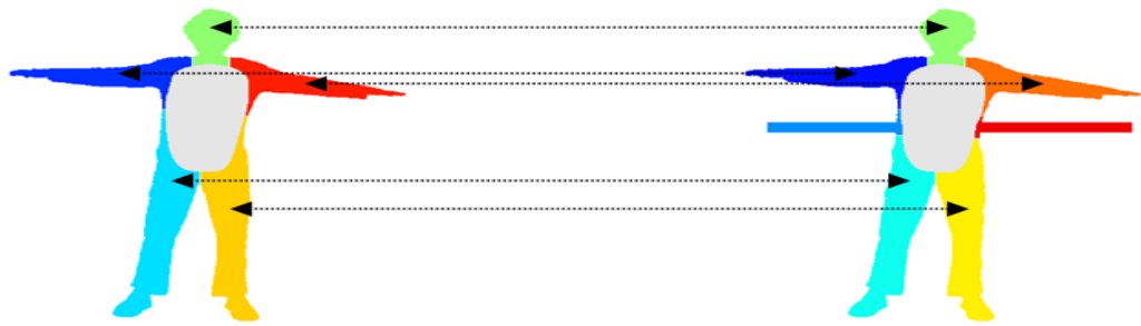
Figure 5.11: (Third example) Matchings between leaf parts of a human shape and its occluded version, whose preliminary part hierarchy trees were given in Figures 5.7 and 5.8.
