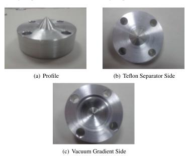
Figure 5.15: The Conical Single Aperture
