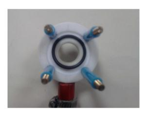
Figure 5.16: The Teflon Separator
