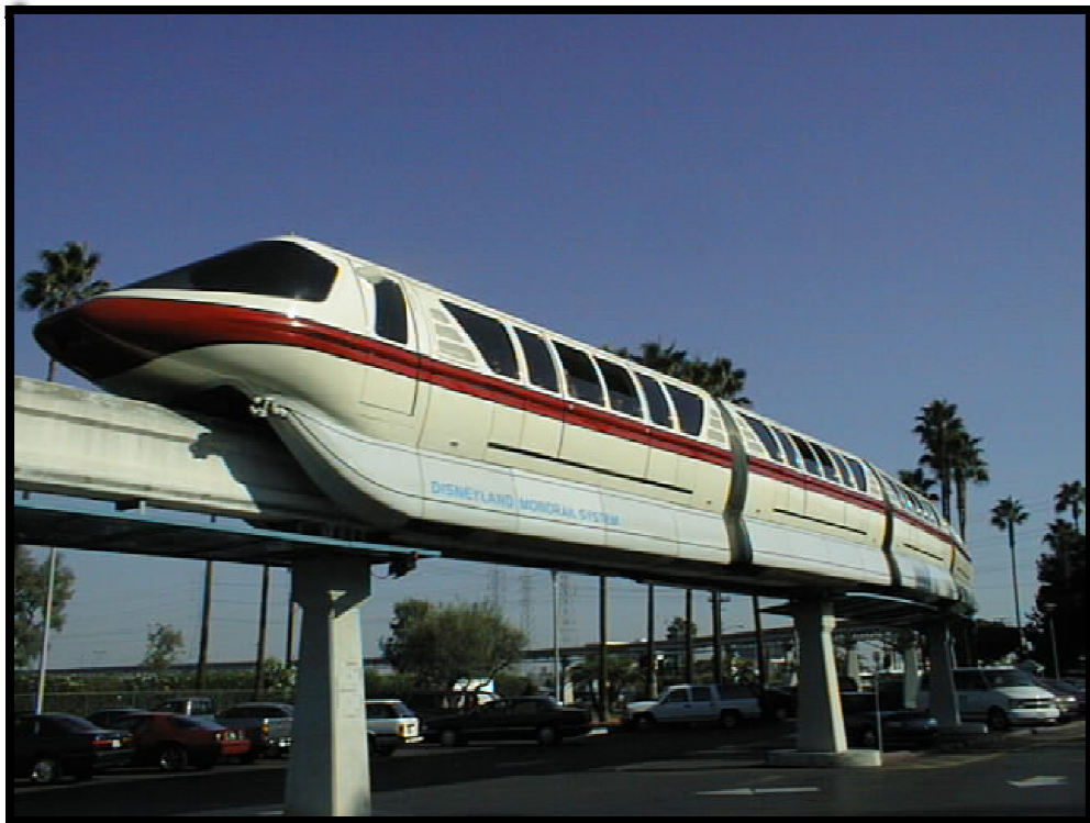
Figure 2.2: Disneyland straddling Monorail Red, Anaheim, CA, USA
