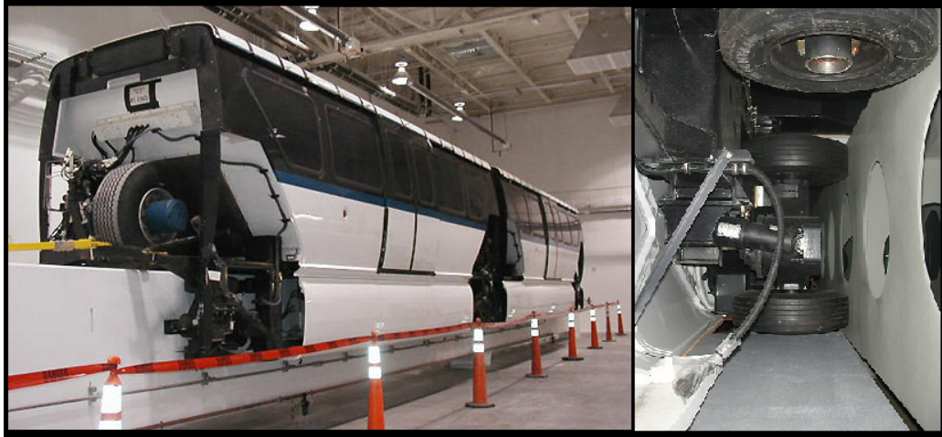
Figure 3.11: monorail's load tires (left) and steering guide tires (right).
