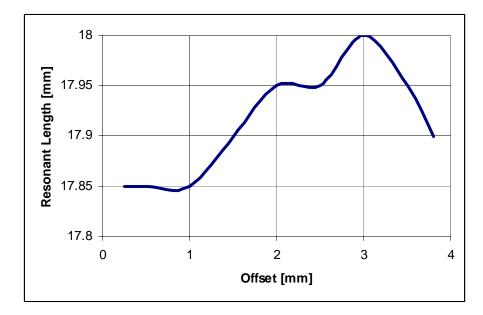
Figure 4.7 Resonant lengths of broad wall slots for various offset values
