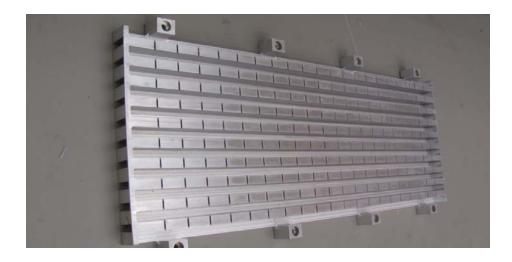
Figure 3.38 The manufactured small edge wall slot array
