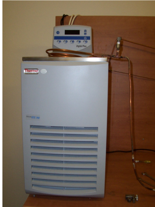
Figure 8: The refrigerant bath and the coil heat exchanger
