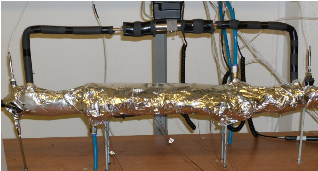
Figure 23: Test section with copper tube after insulation
