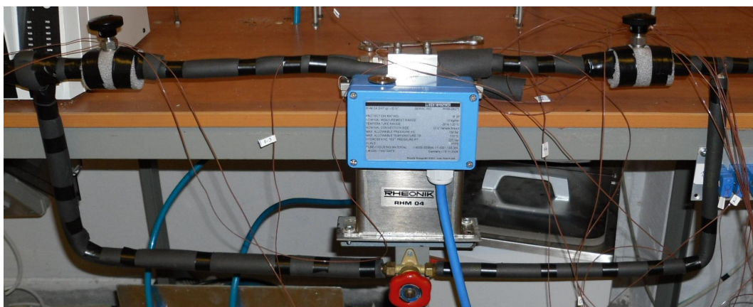
Figure 11: The photo of flowmeter and by-pass line
