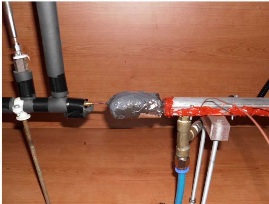
Figure 21: The exit of the test section with solidified glue at the adapter
