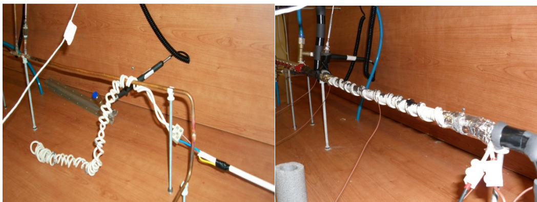
Figure 12: The pre-heater before and after winding
