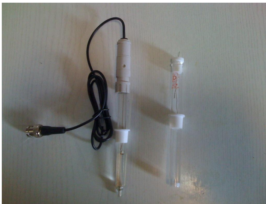
Figure 3.2 Reference electrode (RE) (left) and counter electrode (CE) (right)
