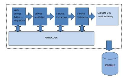
Figure 3.2: Achitecture of Crawler Layer [21]
