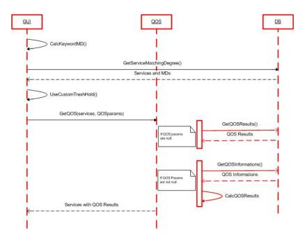
Figure 3.7: Relation between GUI, QoS and DB
