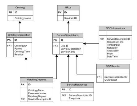
Figure 3.6: Database Architecture
