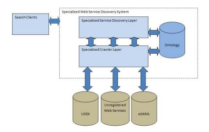
Figure 3.1: The architecture of DSWSD-S [21]
