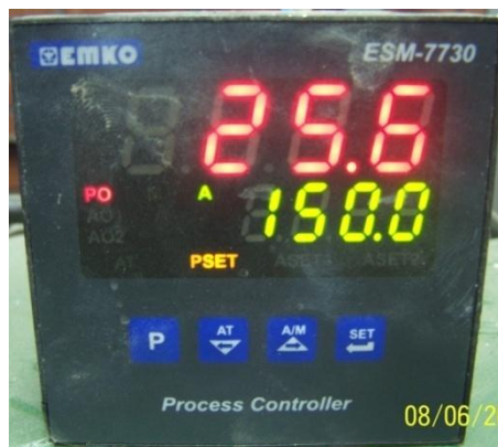
(b) Process controller to maintain the desired load throughout each load step (Step loading)
