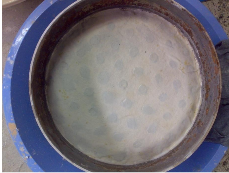
Figure 3.13 The top view after the formation of the piles
