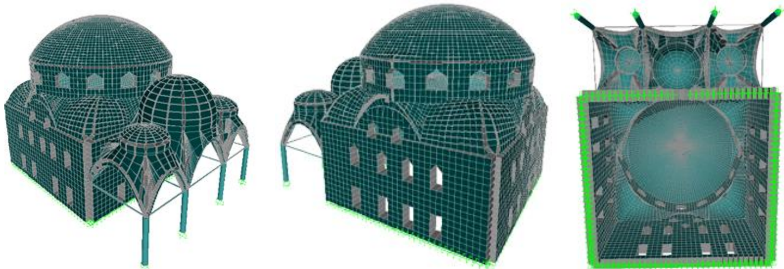
Figure 4.12 Finite Element Model of the structure
