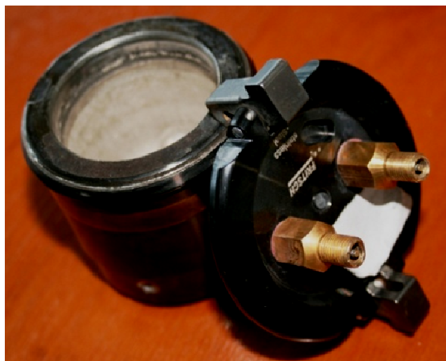
Figure 3.5. Vials used for mechanical milling and reactive milling.
