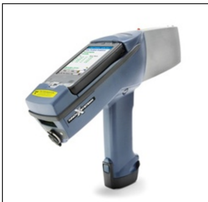
Fig. 12 - The XRF device used for this study. Innov-X Systems Model A-2000 Rhino.
